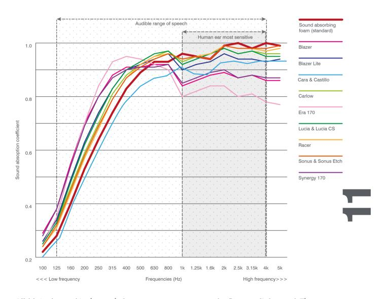
All fabrics featured in the graph demonstrate transparency and reflect very little sound. The sound absorption capabilities of each product vary however according to the frequency of the sound waves:
