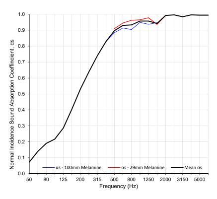
Figure 3: Normal incidence sound absorption coefficient α<sub>S</sub> of the melamine foam.
